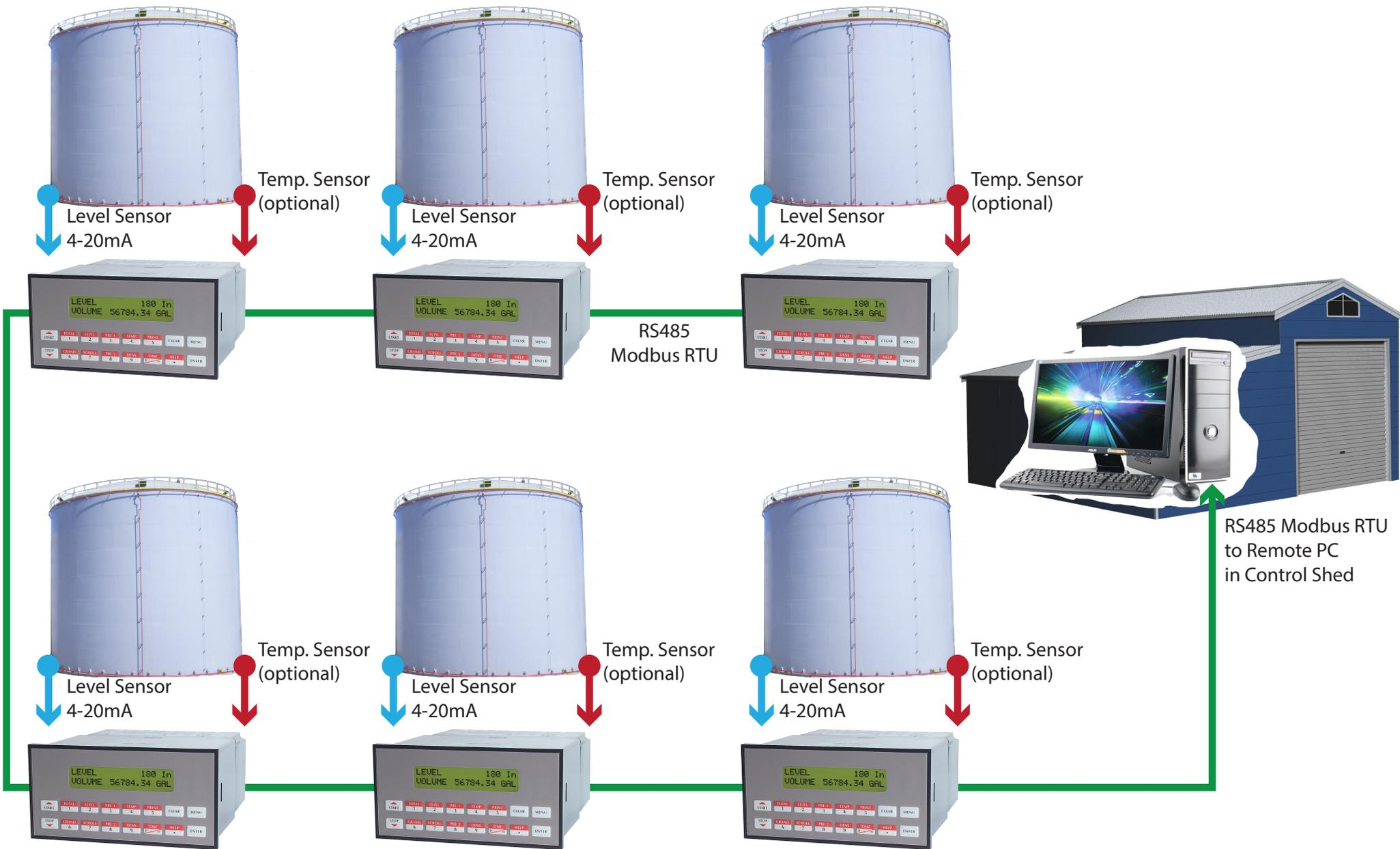
Each tank being monitored is equipped with a level sensor (temperature sensor optional). The level signal from each tank is sent to a LEVELtrol II Level Display Monitor. Each LEVELtrol II is connected to a Modbus RTU network and connected to a remote PC. Information from each LEVELtrol II can be accessed from the PC using TROLLink or Infilink HMI Software.
